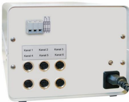
Dosage counter pe6180-X, back view
